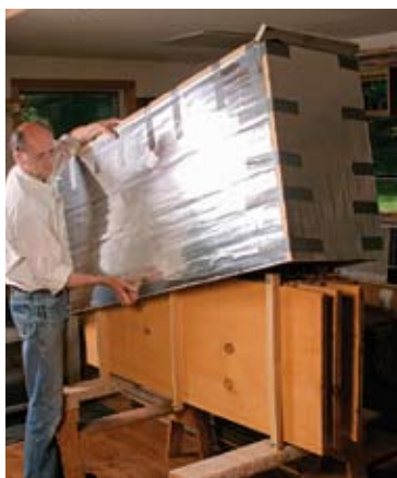
Woodworker's oven. Becksvoort uses a kiln made from foil-faced rigid insulation to cook large pine boards and set the pitch.
